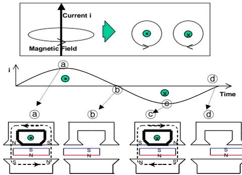
Fig. 5. Operating principle of an oscillating linear motor.
