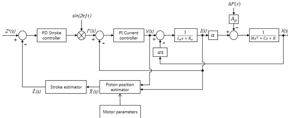
Fig. 6. Block diagram of the closed-loop sensorless stroke control system.
